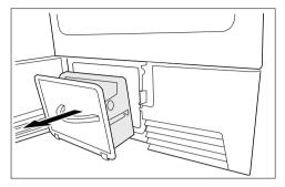
2. Pull the filter housing out of the base by the handle.
